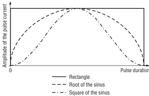
**Figure 2.** Shapes of the tested pacing pulses.
