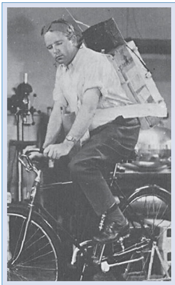
Figure 1. The original Holter device from 1947, weighing 38 kg.
