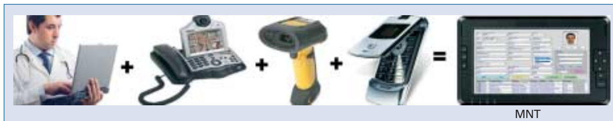
Figure 2. Mobile Nursing Terminal (MNT) (shown in the rightmost panel) combines the features of the notebook computer, video phone, barcode scanner and cell phone. The interactions and data entries are accomplished by voice commands and the touch-screen.
