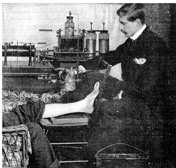
**Figure 2.** 'Photograph of a patient's ankle being skiagraphed together with the apparatus necessary; on the left is seen the induction coil and on the right the Leyden jars and Tesla transformer. The operator controls the key and passes the current at intervals of one-quarter of a minute, so as to give the tube time to cool and to allow the glass to recover from the intense molecular strain'
